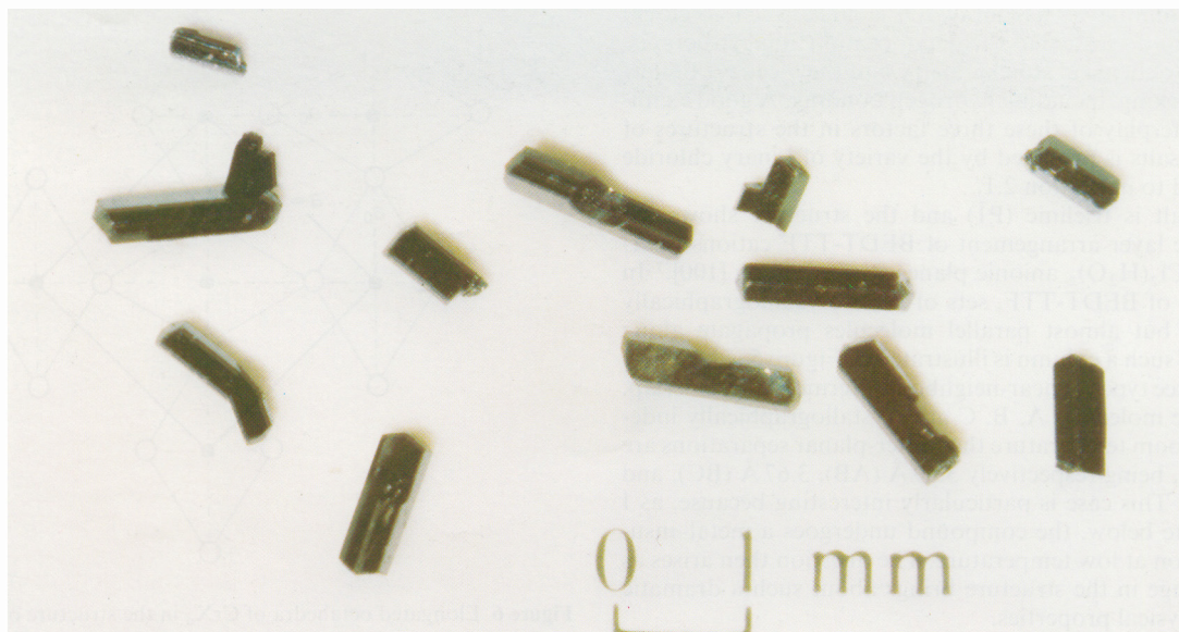
Figure 2 Crystals of \alpha' -(BEDT-TTF) 2 AuBr 2 .
