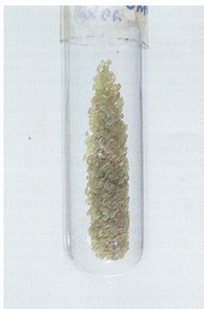
Figure 3 Crystals of (CH 3 NH 3 ) 2 CrCl 4 .
